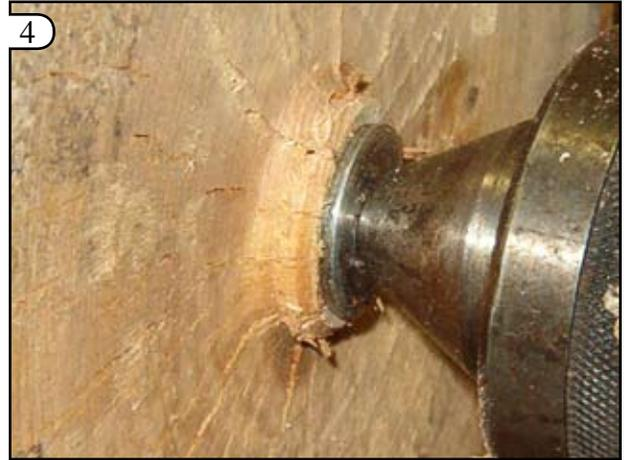
4 Note the washer on the tail stock. I flatten the washer leaving a tenon the size of the washer's diameter. The washer not only prevents the tail stock from digging too far into the piece, it is also selected to be the inside diameter of the face plate. Once the wood is off the lathe the face plate automatically centers on the wood for attachment.
