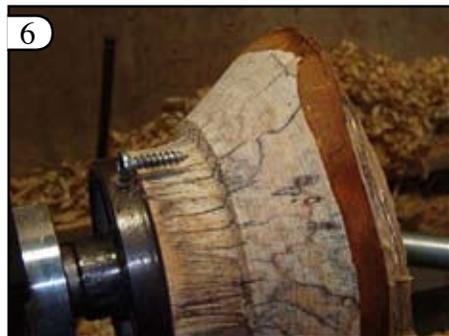
6 First I turn the wood down from the face plate to get past the cracks and to get past the screws for the anticipation of later parting from the lathe.
