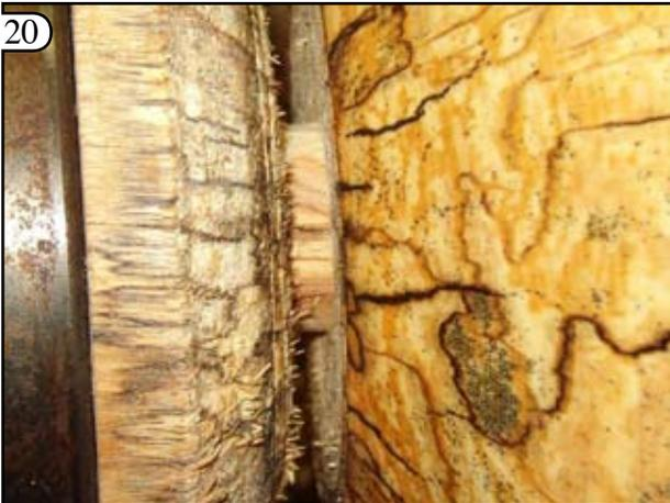
Then the parting tool is used to cut away the tenon and the bowl is cut away from the lathe with a saw. The bottom will be sanded later, after the oil is dry.
