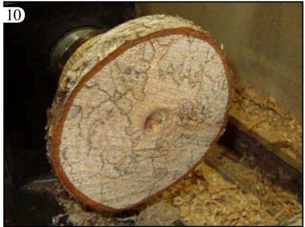
Moving to the top of the bowl, I establish the center and drill a hole to within a half inch of the bottom. I could drill all the way but I like to leave room for changes as necessary. There is no way to know what splits, cracks or other problems may be waiting.
