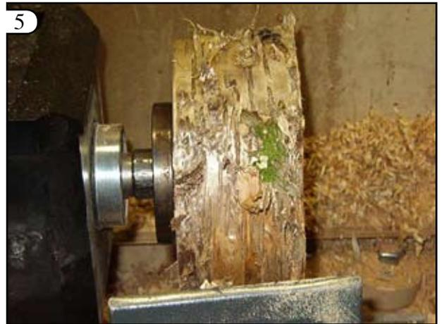
5 The wood is fastened to the face plate with 1" long #14 self tapping sheet metal screws and remounted to the lathe.
