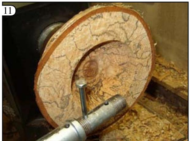
The inside of the bowl is turned away. Even though I use a hook tool for the task, there are few shavings due to the nature of the spalting of this wood.
