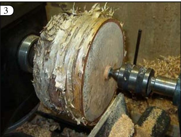
3 First I mount it between centers and flatten the end with all the cracks to receive a face plate.
