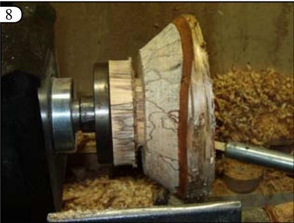
Being far enough in, I part well in to establish the desired bowl bottom. Establishing the diameter helps the eye direct the cutting lines for the final form.
