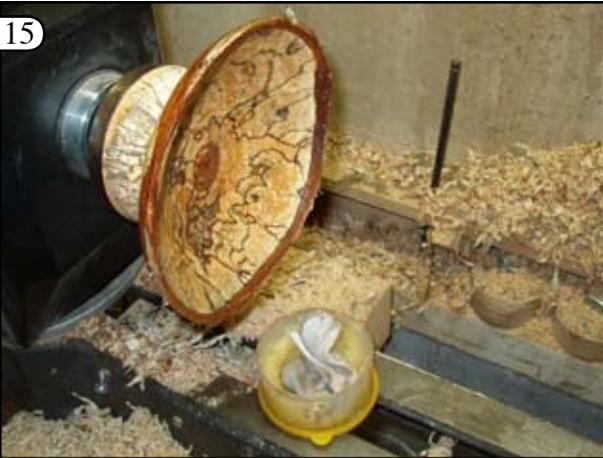
I coat the inside and outside with paste wax to ease the sanding. I have no idea why this helps but I know that the wax will speed up the first sanding immensely. The wax I am using is a blend of 2 parts mineral oil, to 2 parts vegetable oil to 1 part bee's wax. In this case I will start with 60 grit and proceed all the way to 2000.
