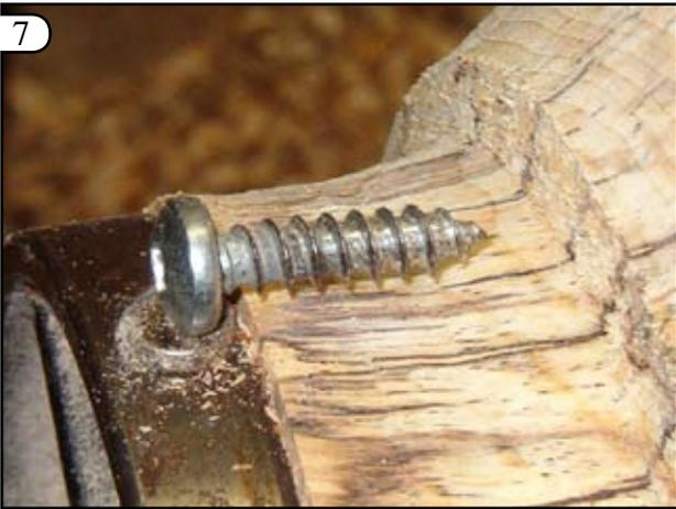
In order to be sure I am far enough from the screw tips to fit in a parting tool, I check the distance with a spare screw I keep by the lathe.
